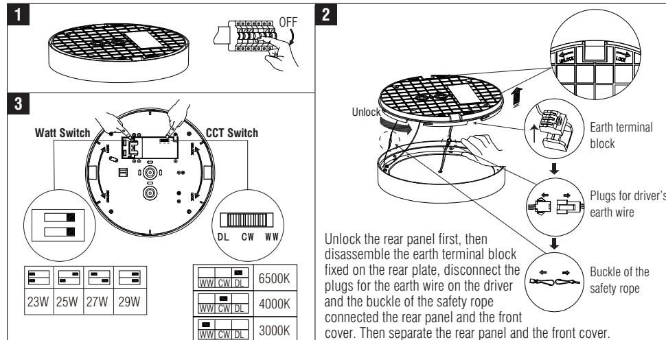
Unlock the rear panel first, then disassemble the earth terminal block fixed on the rear plate, disconnect the plugs for the earth wire on the driver and the buckle of the safety rope connected the rear panel and the front cover. Then separate the rear panel and the front cover.
